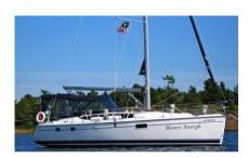
LOA 34' 11" / 10.64 m Beam 12' 4" / 3.76 m 31' 1" / 9.47 m 5' 0" / 1.52 m LWL Draft **Keel Type** Wing keel Rigging Type B&R Fractional Fuel 38 gal / 132 L Water 75 gal / 284 L Waste 30 gal / 114 L Disp 15,328 lbs / 6,953 kg
