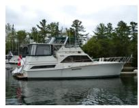
46' 0" 15' 2" LOA Beam 3' 6" Draft Fuel 480 US gal Water 150 US gal Waste 100 US gal 13' 3" Weight 40,000# Clearance 6' 3" Hull Type Modified-V Headroom
