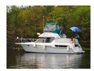
LOA **36' 2"** (w platform) Length 32' 2" 11' 10" Fuel 168 Gallons (2 x 84) Beam 35" 51 Gallons Draft Water 6' 2" Headroom **Holding tank 20 Gallons** Sleeps Weight **15,100#** (w/fuel & water) 6
