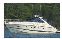
LOA 57' 0" w/platform Beam 14' 5" 3' 8" Draft Fuel 465 gal Water 130 gals. Weight 42,460# 6' 2" 12' 9" Headroom Clearance
