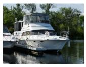
39' 9" 14' 3" LOA Beam Fuel 400 gallons Draft 3' 8" Water 150 gallons Waste 55 gallons Weight 19000 lbs Deadrise Aft 12°
