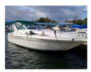
29' 9" LOA 31' 11" (w/pulpit) LOH Beam 10' 6" Fuel 120 gallons 2'8" 35 gallons Draft Water Waste 28 gallons Weight 8300 lbs Deadrise Aft 21° Sleeps
