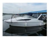
9' 7" 30' 3" LOA Beam 2' 1" Draft down 3' 5" Draft up 109 gallons Water Fuel 33 gallons Waste 13 gallons Weight 8,056 lbs
