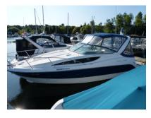
LOA 28' 9" (w/extended platform) Draft 37" (20" drive up) Fuel 102 gallons Waste 20 gallons Sleeps 6 Beam 9' 10" Deadrise 17 deg. Water 33 gallons Weight 7241 lbs
